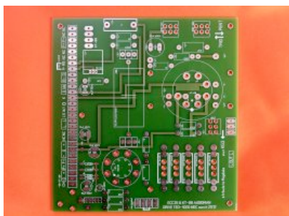
driver PCB I developed to enable A2 operation
