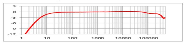
Bandwidth for various Rgen RL=100K //100pF, secondary grounded
