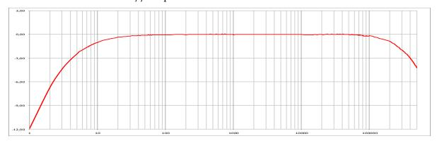
Bandwidth for various Rgen RL=100K //50pF, secondary grounded
