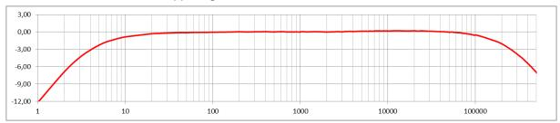
Bandwidth for various Rgen RL=100K //50pF, secondary grounded
